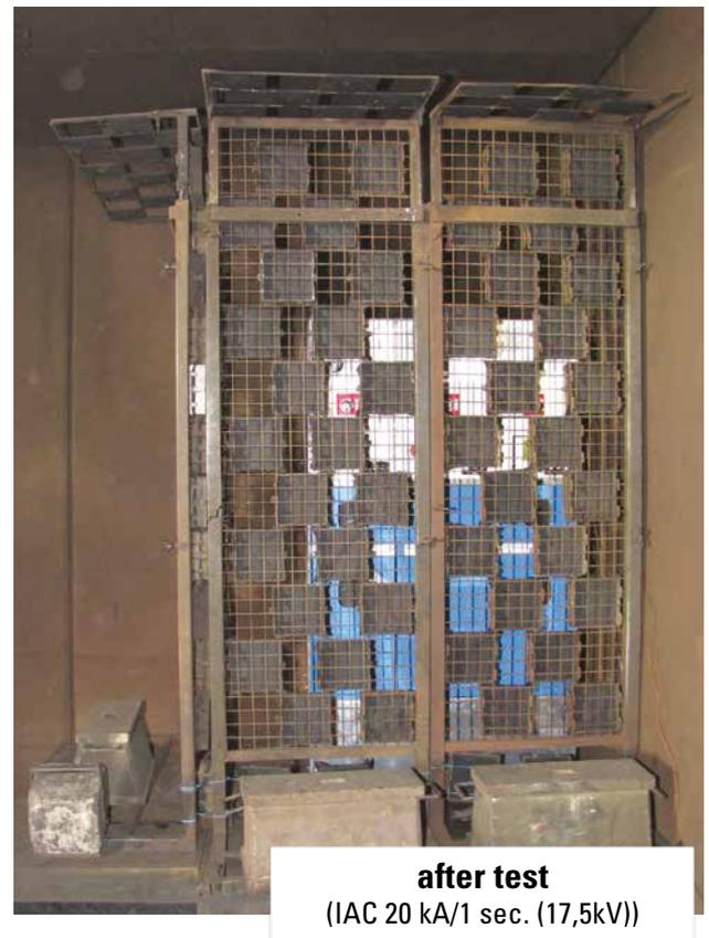
*The various tests were always in accordance with IAC (AFL) for 16kA/1s. according to IEC 62271-200*
